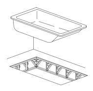
Install Using Gypsum: Place a 2" thick layer of gypsum cement (such as Gyp-Crete 2000) on the floor where the whirlpool is to be set. This will help secure, level and support the bath. Set bath into position. Clear any excess cement from vicinity of the pump.
